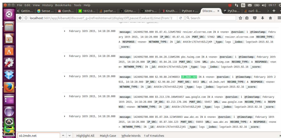
Figure 4.6: Indexed DNS log after being processed by Logstash tool and stored in the ES , and it is shown using the tool for searching and data visualization called Kibana . The queried URL is s0.2mdn.net .
