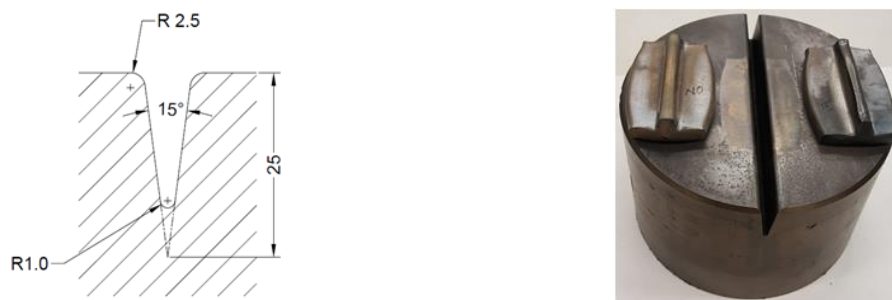
Fig. 6.1: (left) The sectional shape of die, (right) experimental grooved die together with deformed specimen
