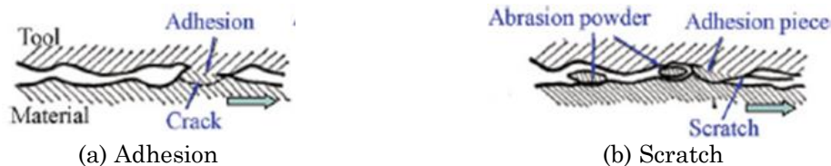
Fig. 2.27: Schematic of disadvantages of using improper lubricants [GHA15]
