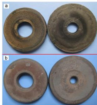
Fig. 2.34: Samples deformed at 30% and 50% height reduction: (a) glass lubricant and (b) dry friction [ZHU11]
