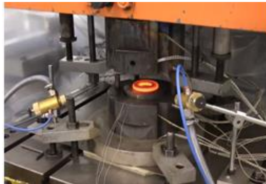
Fig. 5.2: Experimental set up with the water-graphite lubricant spraying system
