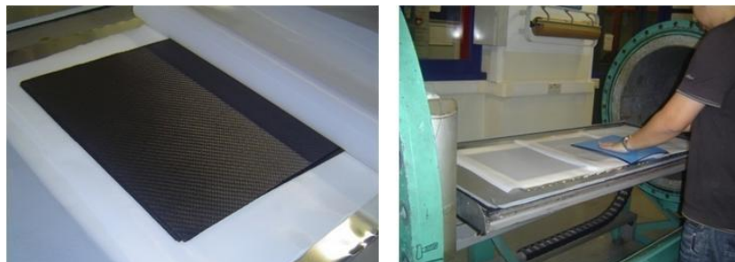
Figure 26: Manufacturing process in the autoclave in KU Leuven facilities
