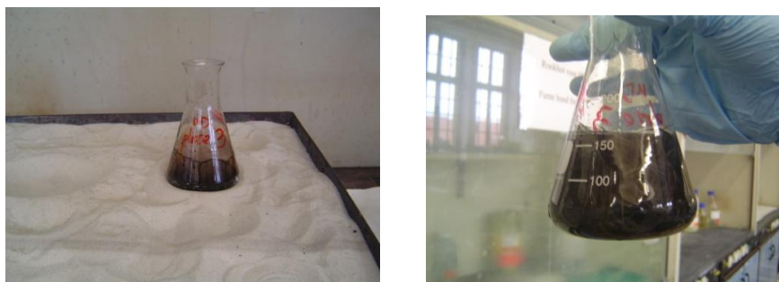
Figure 27: Sample with the acid for at least 20 minutes on the sand oven for removing the matrix
