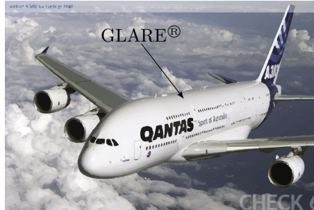
Figure 2.2: Image of the Airbus A380 highlighting the upper fuselage which is made of GLARE®.
