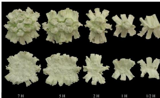
Figure 10. Bottom and top views of post-crushed specimens for all the configurations.
