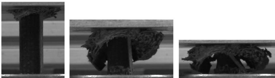
Fig. 4. [Bas]<sub>8</sub> configuration. (a) Progressive initial crushing process. (b) Collapse of the base section. (c) Buckling and loose of properties of the specimen.
