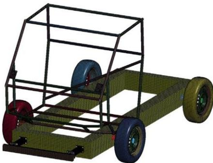
Figure 8. FEM model for the structure of the L7e vehicle prototype.
