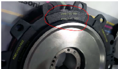
Fig. 8. Friction disc of the clutch brake. Friction pad is highlighted by a red circumference.
