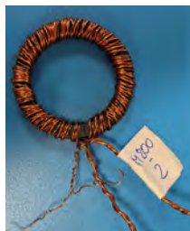
Figure 3.10: Laminated toroidal core made of electric sheets of grade M800-65A.
