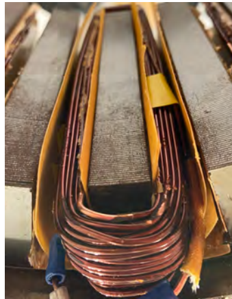
Figure 5.22: Coil with 3 liner layers of 0.3 mm each.
