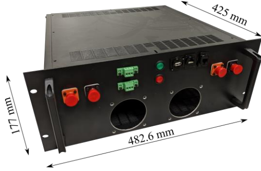
Fig. 10. Image of the assembled 19 inch rack.
