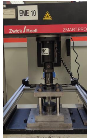
Fig. 3-14 Zwick 050TM universal testing machine (depicting a test specimen during testing).
