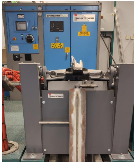
Fig. 3-3 Inductotherm induction furnace.
