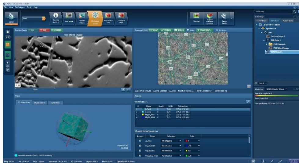
Fig. 3-13 Interface of the AZtechKL acquisition and analysis software; The (SrZn 13 ) phase is identified from the candidate list using electron backscatter diffraction pattern (EBSP). This sample corresponds to the Sr and Sb modified alloy detailed in Chapter 6.
