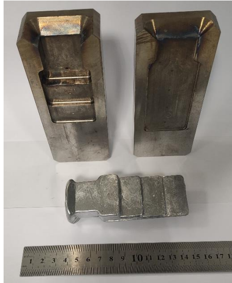
Fig. 3-2 Stepped mold made of AISI H13 steel (Total volume: 29,177 mm 3 ).
