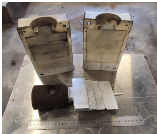
Fig. 3-4 Stepped mold made of AISI H13 steel (Total volume: 141,547 mm 3 ).
