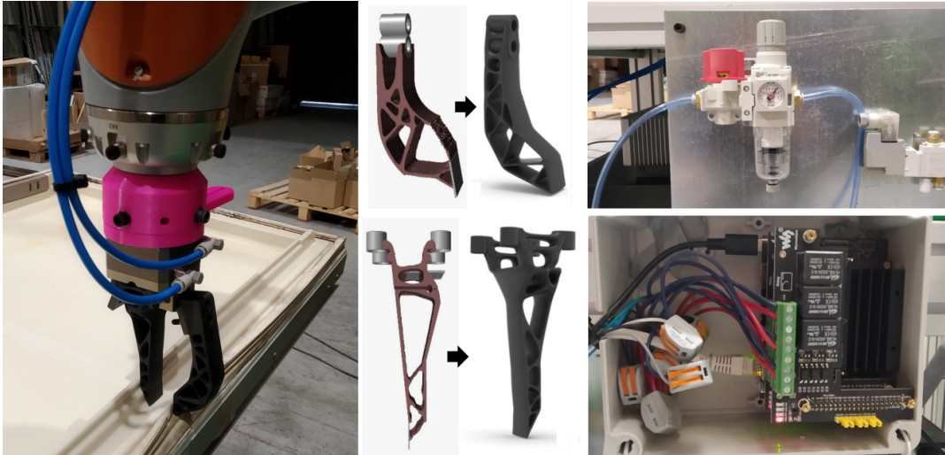
FIGURE 8.3: A pneumatic gripper with generative designed fingers printed using additive manufacturing for disassembly and its control system.
