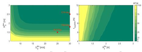
(a) Overall WT sensitivity:  $U_w^{lim}$  vs.  $H_s^{lim}$ . (b) Overall WT sensitivity:  $H_s^{lim}$  vs.  $t_{reqWW}$ .
