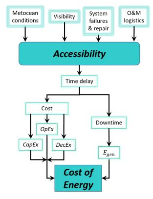
Figure 1. Schematic diagram of accessibility.
