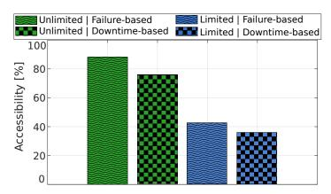
**Figure 6.** Comparison of the failure- and downtime-based accessibility metrics for the GEROA wind farm.
