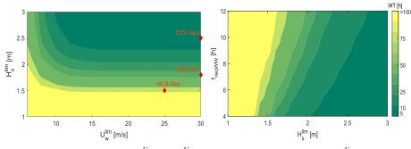
(e) Winter WT sensitivity:  $U_w^{lim}$  vs.  $H_s^{lim}$ . (f) Winter WT sensitivity:  $H_s^{lim}$  vs.  $t_{reqWW}$ .
