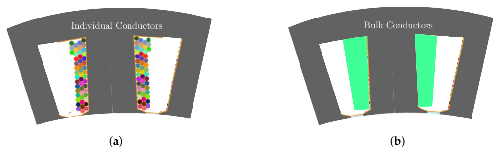
Figure 3. Magnetodynamic models: (a) full; (b) simplified.
