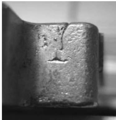
Figure 2.11: Cold shuts (Adapted from Janudom et al., 2010)
