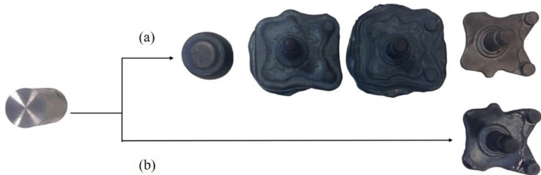
Figure 2.3: (a) classical hot forging (b) NSF process in the case of a H spindle geometry (Lozares et al., 2020)
