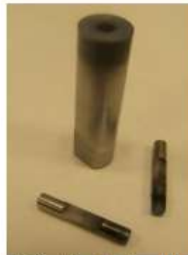
Figure 1: Modular tool used for FSW.
