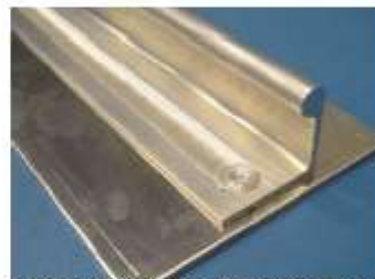
Figure 4: Detail of the end of the FSW joint.
