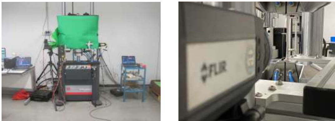
Figure 70: Setup for the fatigue tests monitored by IR thermographic cameras.
