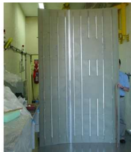
Figure 11: Reinforced panel manufactured by FSW stringer-skin lap joints and skin-skin butt joints [22].
