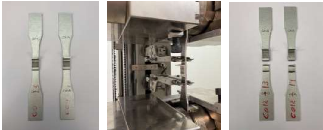
Figure 69: Specimens machined from coupons C3 (left); C6 (right); and the setup for the static tensile tests (middle).
