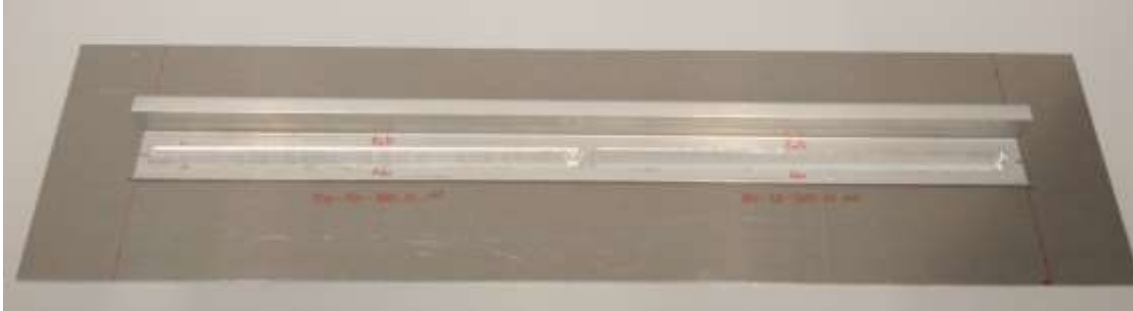
Figure 86: FSLW joint-coupon manufactured using a AA2198-T8 sheet/skin and a AA2196-T8511 extrusion/stringer.
