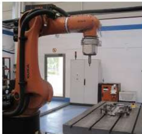
Figure 1: Robotic FSW system at IK4 LORTEK used for FSW tests.
