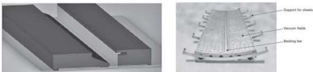
Figure 20: Clamping systems for FSW: Z-stringer clamping – courtesy of MTS (left); Vacuum clamping fixture – Courtesy of Airbus-Bremen (right), [33].
