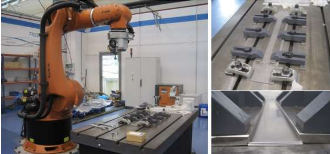
Figure 91: Robotic FSW system used for FSLW tests using AA2198-T8 sheets of small thicknesses.
