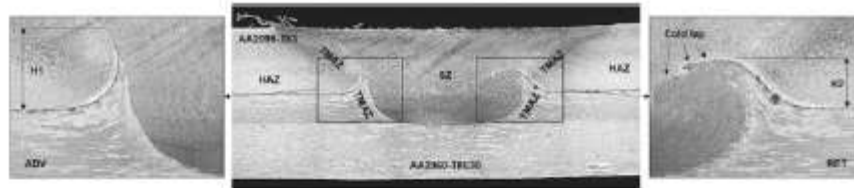
Fig. 3 Cross-section of FSW lap joint produced at 1200 rpm and 250 mm/min by a conventional threaded tool
