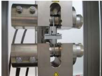
Figure 6: Special jig for pull-out testing clamped in the tensile testing machine.
