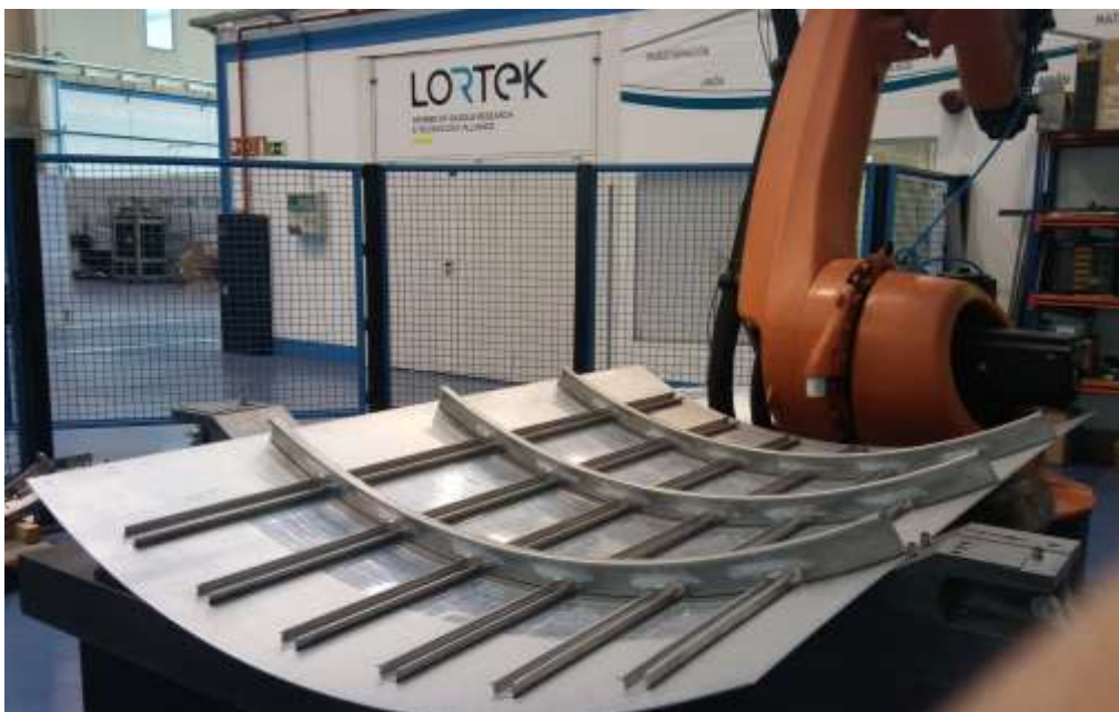
Figure 96: Initial fuselage panel demonstrator manufactured in the robotic FSW system at LORTEK.
