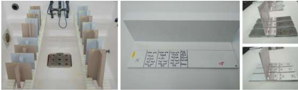
Figure 84: Disposition of the FSLW joint-coupons in the NSS chamber during the ASTM-B117 NSS corrosion test (left); FSLW joint-coupon 4 after NSS exposure (middle); and specimens cut from FSLW joint-coupons ready for static pull-out tests (right).
