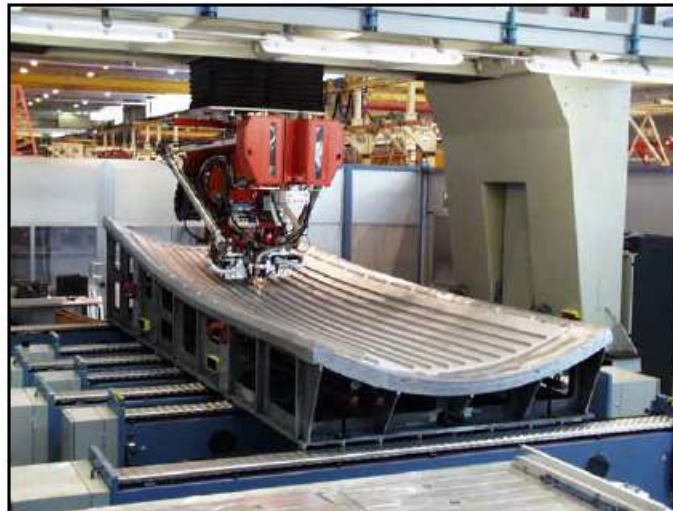
Figure 8: LBW facility at Airbus [15].
