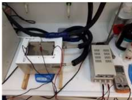
Figure 1. Experimental setup for the thin film sulphuric acid anodising (TFSAA) alongside TFSAA process parameters.
