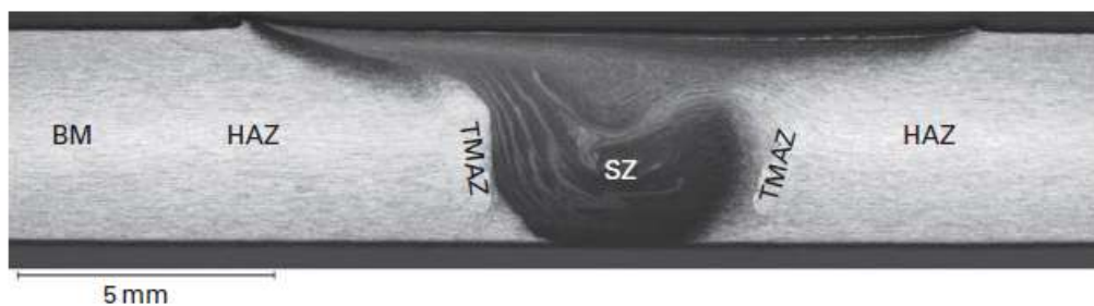
Figure 18: Transversal section of a Al-Mg-Sc FSW joint showing the typical microstructural zones in FSW [33].
