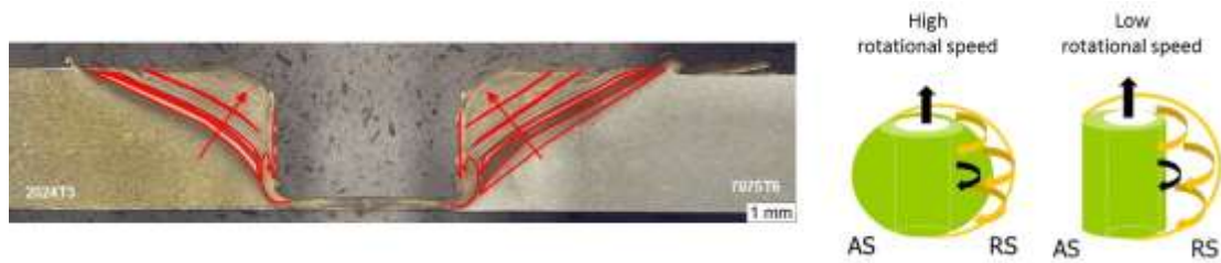
Figure 16: Material flow pattern during FSSW for threaded probes and different rotational speeds [43] [44].
