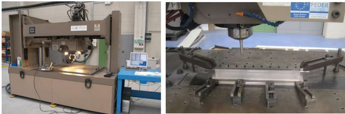
Figure 50: i-STIR PDS 4 FSW machine used for FSW manufacturing tests (left); clamping configuration developed to produce the FSW coupons using AA2099-T83 extrusions on top of AA2060-T8E30 sheets (right).
