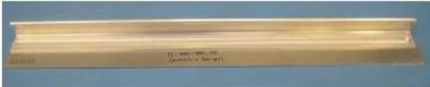
Figure 2: Part produced by stringer-skin FSW.
