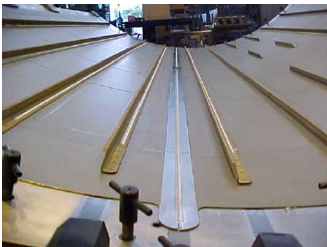
Figure 11: Reinforced panel manufactured by FSW stringer-skin lap joints and skin-skin butt joints [22].
