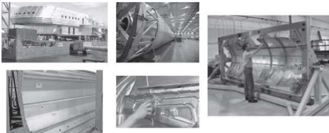
Figure 21: FSW applications for different industry sectors: FSW module for “Finnmarken” at Marine Aluminium (top-left); FSW in a Falcon 9 tank of SpaceX (top-middle); FSW side panels made by Sapa and used by Bombardier (bottom-left); FSW taylor welded blank for BMW and Land Rover (bottom-middle); Lower fuselage reinforced panel made by stringer-skin FSW at Eclipse Aviation (right), [33].
