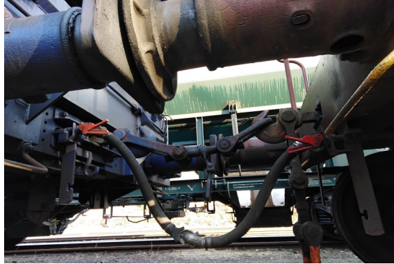
Figure 3.6: Trains manual coupling process.
