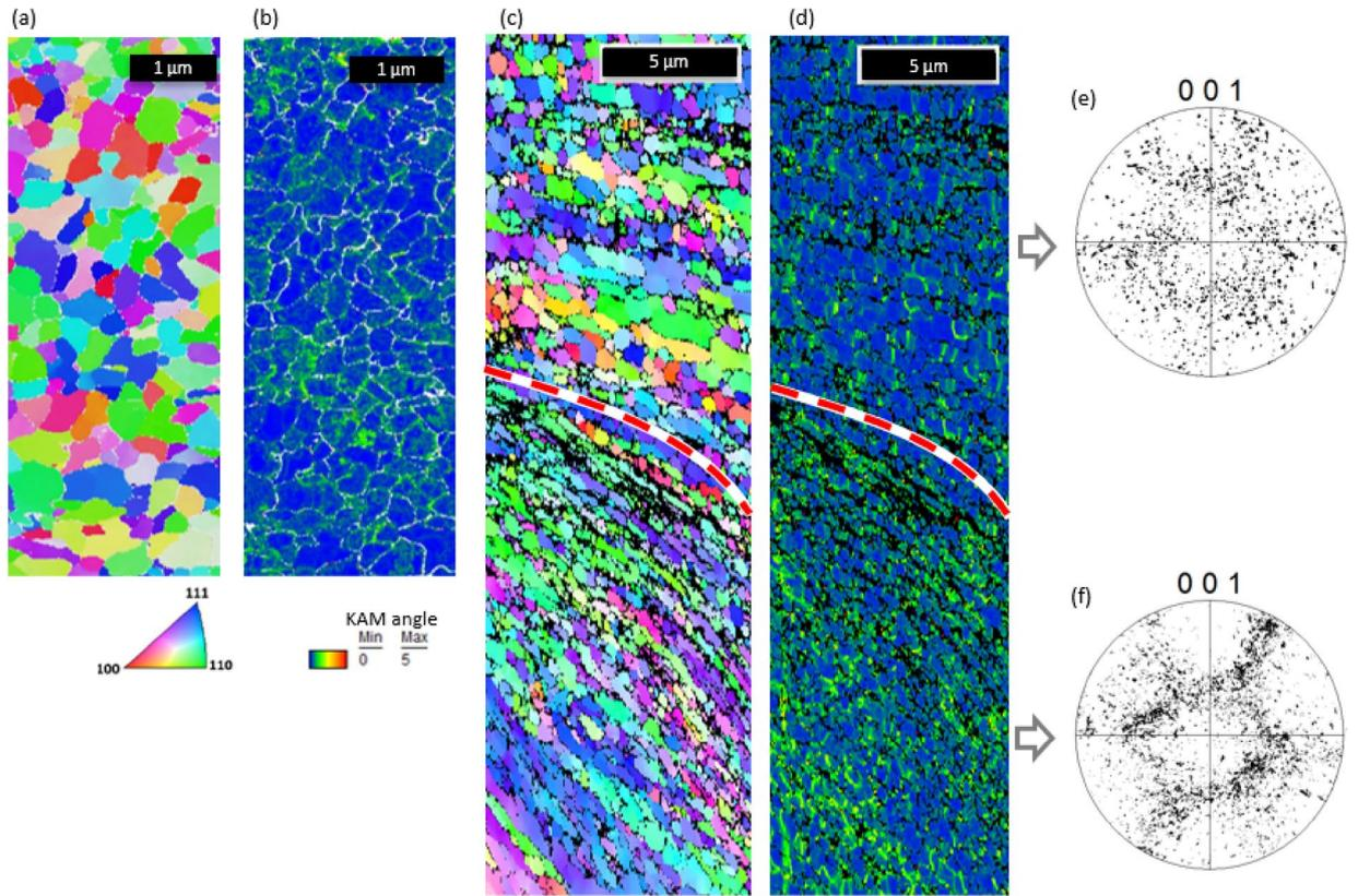
**Figure 3.** Crystallographic orientation by EBSD on frictioning surface (top corresponds to chip-tool contact surface) on chips cut at 200 m/min. (a) Inverse pole figure (IPF) colored in the proximity of the surface and (b) corresponding Kernel average misorientation (KAM) map. (c) IPF and (d) KAM of the whole area affected by friction. (e) and (f) are pole figures (PF) of the area inside and outside of the DRX layer respectively.
