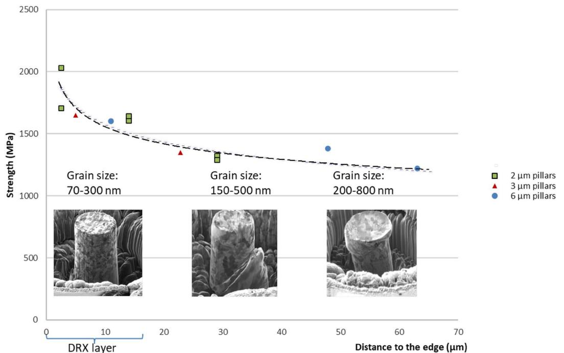
**Figure 4.** Strength values obtained by pillar compression tests of the pillars of 2, 3 and 6 μm of diameter milled on a cross-section at different depth into the material. Pillar diameter does not have notable influence, however pillar closer to the edge show larger strength.
