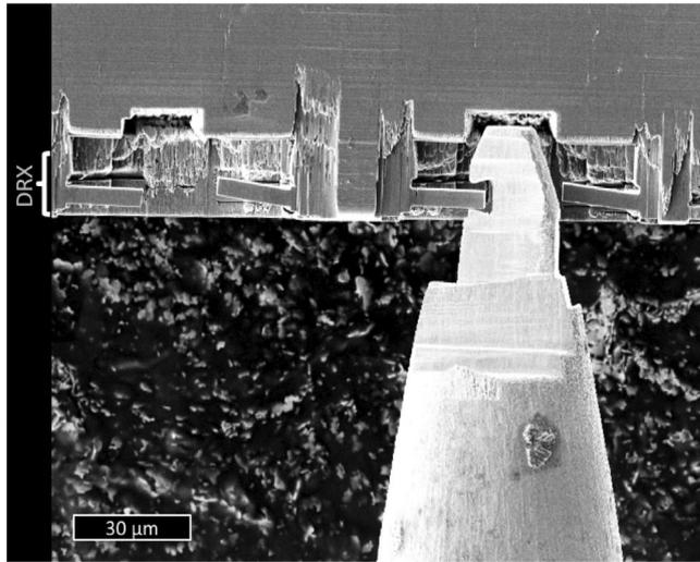
**Figure 8.** Set-up for beam bending in-situ in the SEM experiments. Tip has been fabricated by FIB milling of a tungsten needle.
