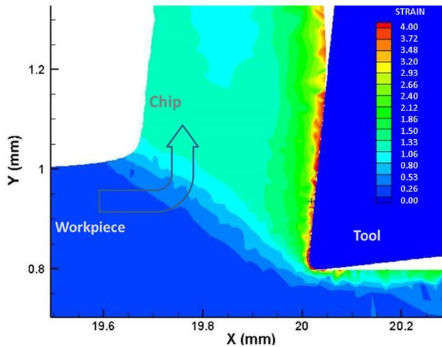
**Figure 9.** Calculations of the strain in workpiece and chip for a AISI 1045 steel cut at 200 m/min and uncut chip thickness of 0.2 mm.
