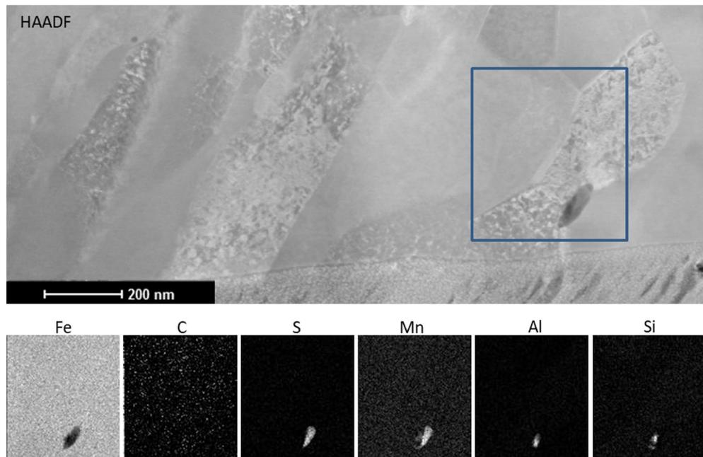
**Figure 2.** STEM-HAADF image of the DRX area (top). EDX chemical maps (bottom row) of the square in the HAADF image depict the distribution of Fe, C, S, Mn, Al and Si. C is equally distributed and does not show excess neither in the inclusion nor in the grain boundaries. Elements typical for impurities in commercial steels constitute the inclusion.
