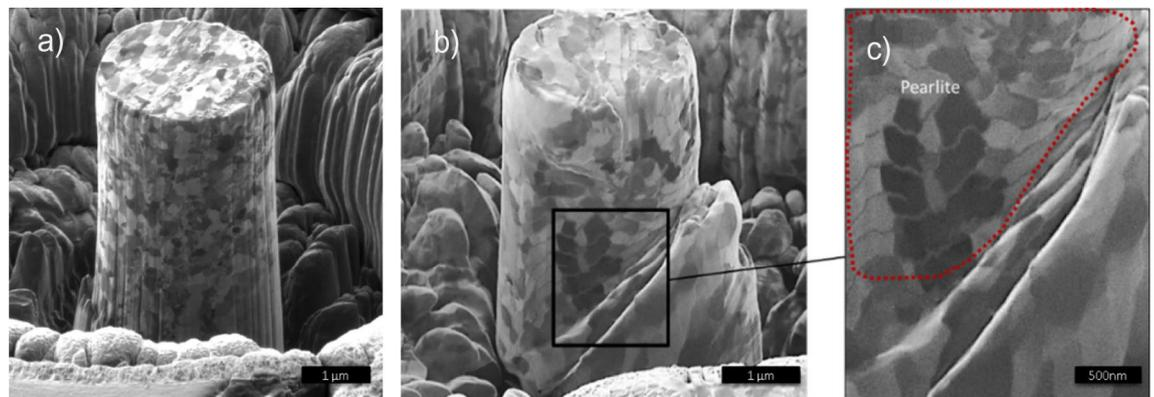
**Figure 6.** A pillar (FIB-scanning) image to reveal the grain distribution and the position of pearlite lamellae, locating the area of shear in the interface between ferrite and pearlite. Nanograined steel (a) depicts a homogeneous deformation, while in for larger grains the boundary of pearlite colonies (b) concentrates the shearing (c).
