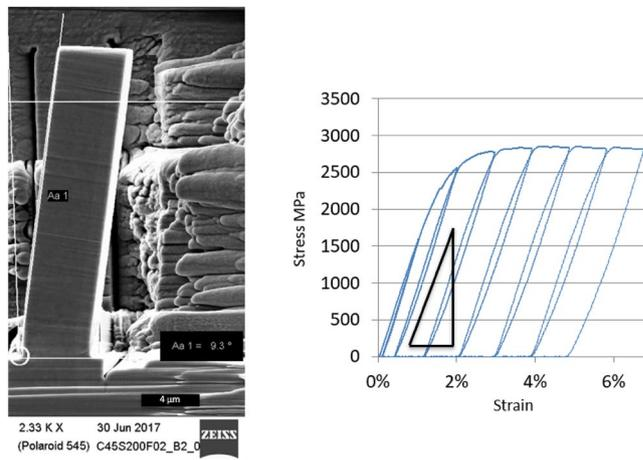
**Figure 7.** Beam bending experiments for elastic modulus calculation. Left: an SEM image of the bent beam after experiment; right: typical measured strain–stress curve for bending experiment.
