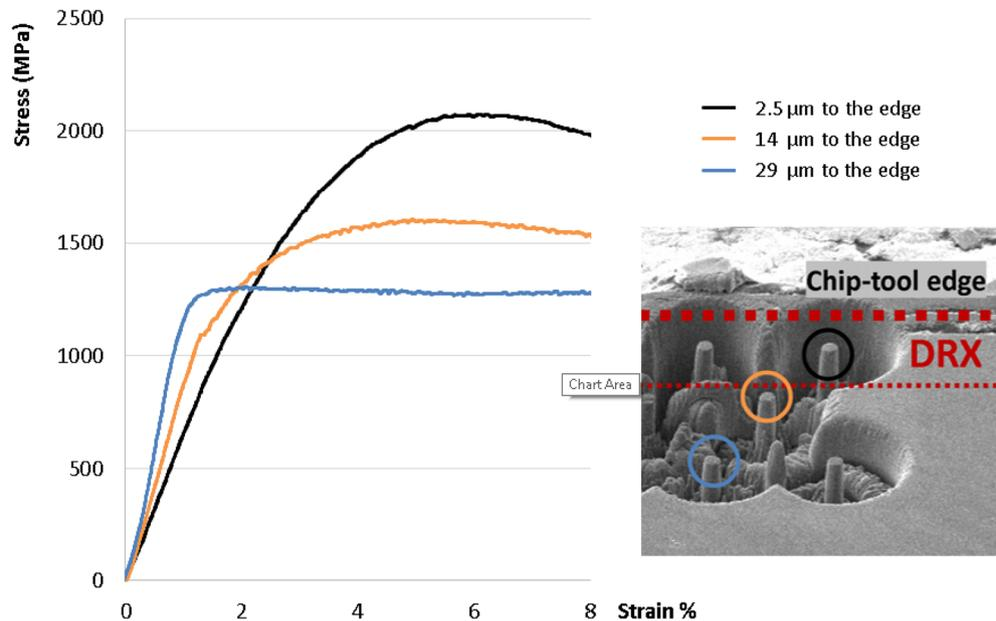
**Figure 5.** The graph shows the stress–strain plot for 2  $\mu\text{m}$  diameter pillars milled at 2.5, 14 and 29  $\mu\text{m}$  from the chip edge.
