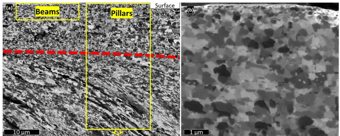
**Figure 1.** Ion image of the chip cross-section machined at 200 m/min. (a) Red dashed line is an estimation of PSZ-SSZ boundary. (b) Detail of the SSZ by ion scanning of chip cross-section when machining at 200 m/min. Crystals tend to equiaxiality and the diameter is consistently in the sub-micrometer range.
