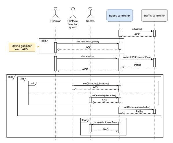
Figure 2. AGV navigation sequence diagram.
