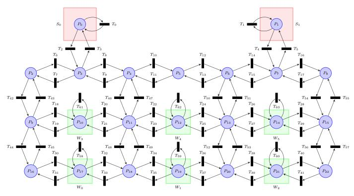
Figure 3. Petri net model of the manufacturing facility.
