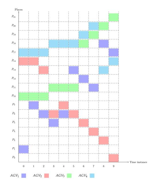
Figure 6. Simulation output: places held by the AGVs in each time instance.
