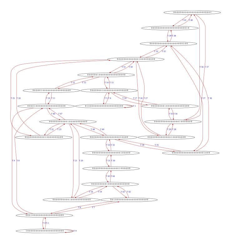
Figure 4. Example reachability graph for a single AGV for the CPN model shown in Figure 3.
