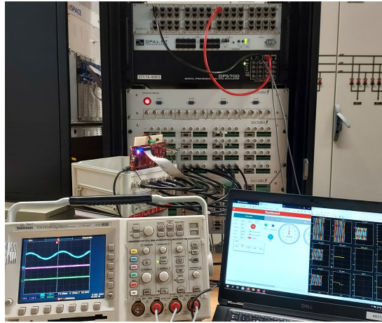
Fig. 19: Opal-RT based real-time HIL testbed.
