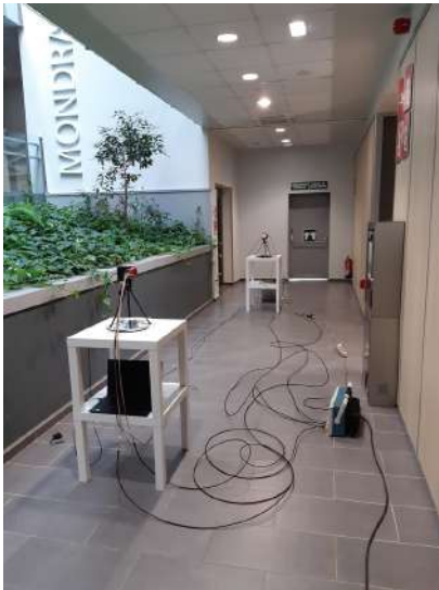
Fig. 5: Delay and power testing in corridor
