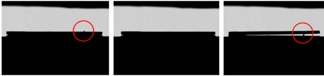
Figure 5.20: Local big burr upwards, correct part and local big burr downwards.
