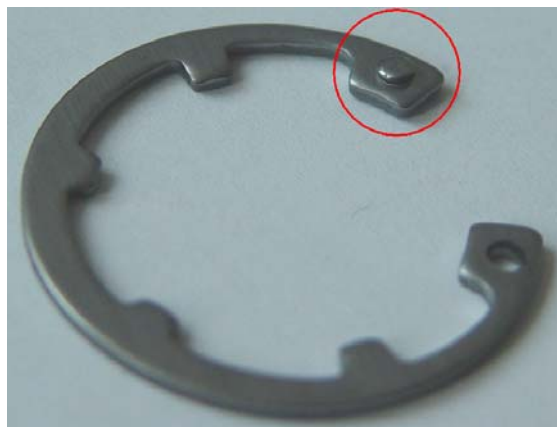
Figure 4.27: Part produced with a punch broken inside the tool.
