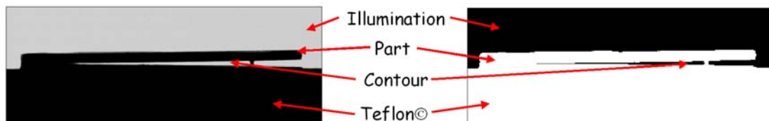
Figure 5.23: Contour detection between the part and the Teflon ® surface.
