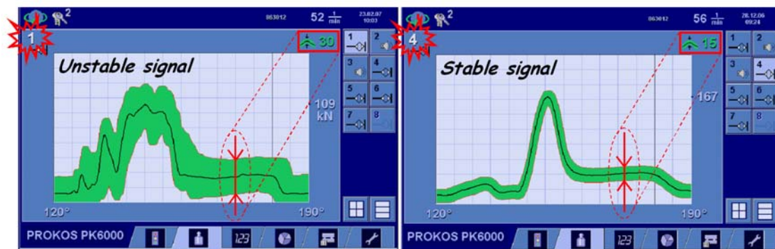
Figure 4.2: Sensitivity set up at Brankamp PK550 unit.
