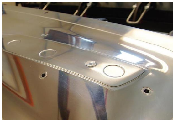
Figure 1-3: Pressure transducer for mold filling detection [Legault 2015 ].
