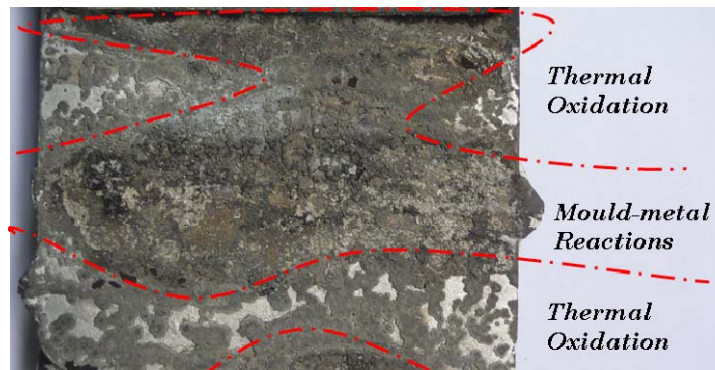
Figure 5.2: Image of the Mg-KL-4mm step, where mould-metal reactions and thermal oxidation zones are clearly distinguished
