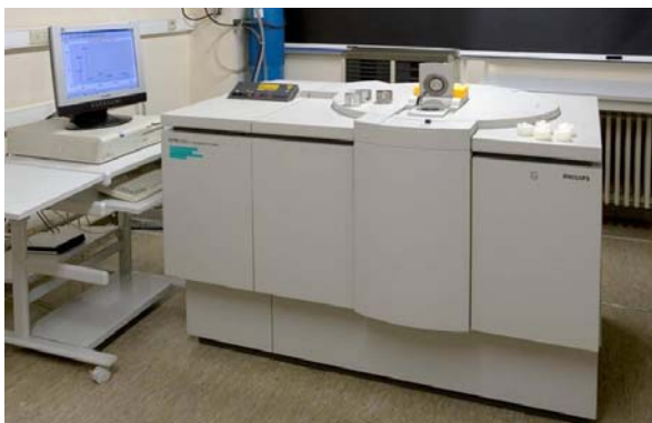
Figure 3.6: Philips PW 2400 automatic sequential wavelength dispersive X-ray fluorescence spectrometer (WD-XRF) at MTM-KULeuven
