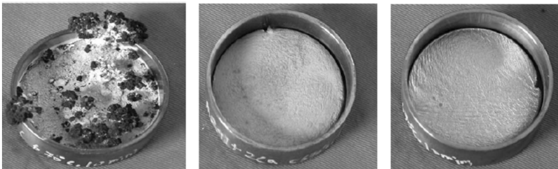
Figure 2.24: Surface s after the oxidation treatment of: a) AZ91 b) AZ91-2Ca c) AZ91-2Ca-0.06Be [Cho06]
