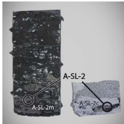
Figure 4.23: Steps obtained in the A-SH casting. Most of the shell was destroyed during its removal
