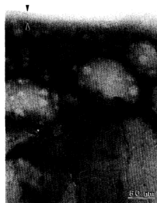
Figure 2.2: Cross view of a film obtained after Mg exposure to humid environment. The film exhibits a duplex structure with a dense amorphous outer layer (black arrows) and a hydroxide inner layer [Nor97]
