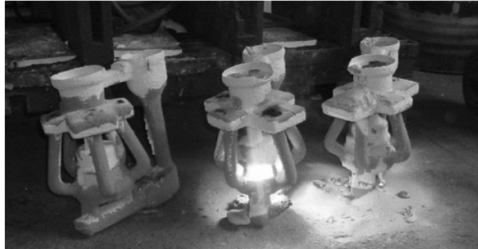
Figure 2.30: Investment casting mould burning due to severe mould-metal reactions [Arr07]
