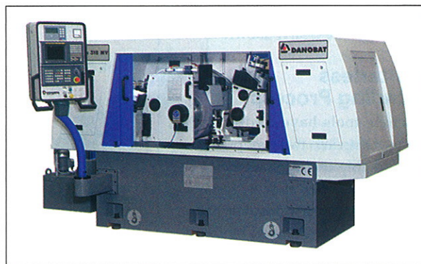
Fig. 4. Centerless grinder machine. In cylindrical grinder machines the workpiece rotates and the cutting device is a grinding wheel. The difference between a centerless machine and a conventional one is that in the former the workpiece is not clamped and a regulating wheel transmits the rotation to the workpiece.
