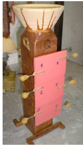
Figure 2. Wax model of the mould. 2 thermocouples have been placed in each step
