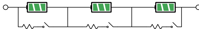
Figure 2.4: Dissipative cell balancing circuit. The excess energy is dissipated by the resistors.
