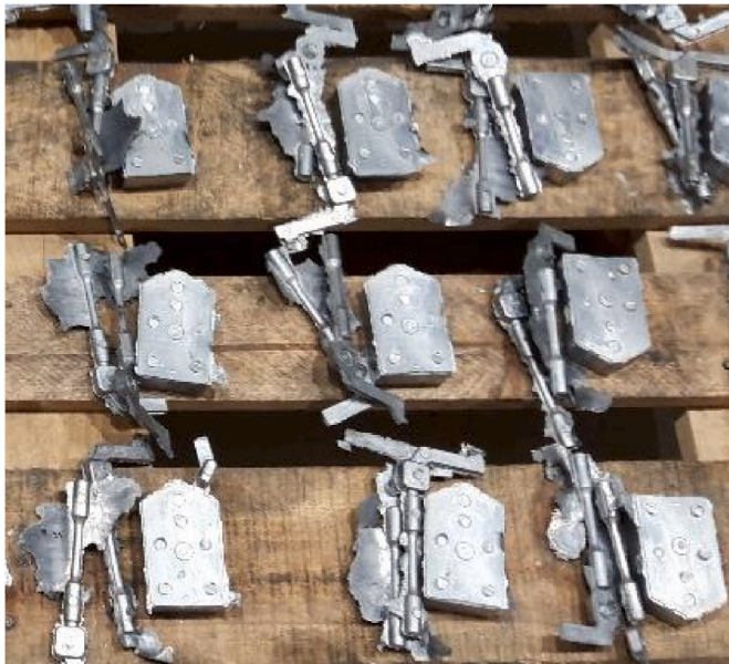
Fig. 2. Example of tensile bars and other testing samples.
