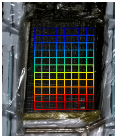
Fig. 6. Grid of ROIs defined on the HSI acquisition of the entire composite part for model prediction.
