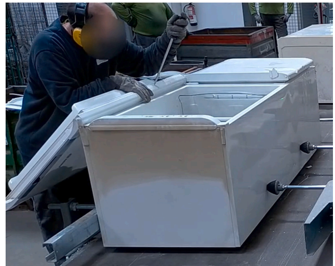
Fig. 8. Magnetic gasket extraction in an actual disassembly plant. The worker uses a screwdriver to pry the gasket slightly and pull it out.
