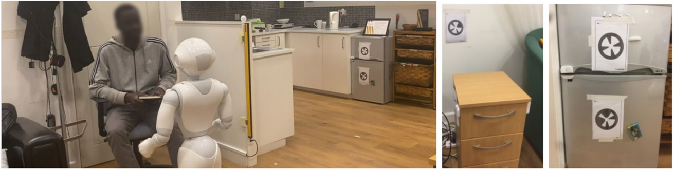
Fig. 1 The AAL studio consists of a living and kitchen area equipped with contact sensors and markers on items such as the medication cabinet and fridge
