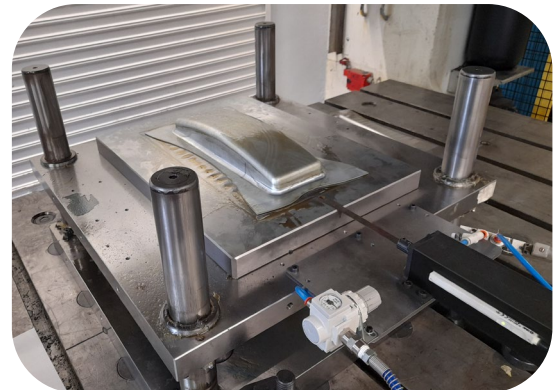
Fig. 6. New sensor assembly in a real deep drawing tooling.
