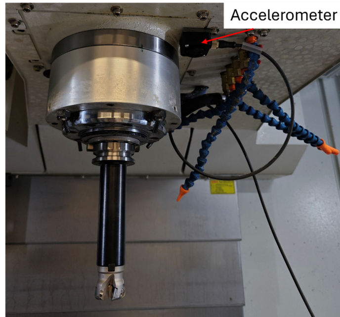
Figure 7. Accelerometer placed on the machine, near the tool.
