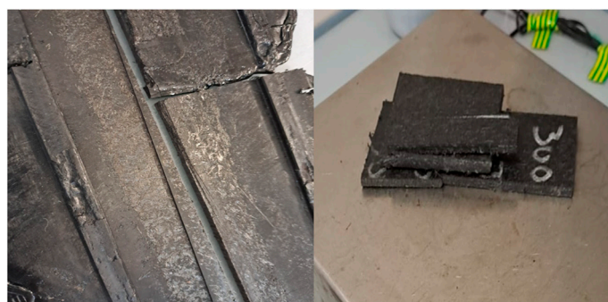
Figure 1. Glass mat-reinforced polyamide-6 composite ( left , as received; right , cuts for experiments).
