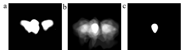
Fig. 7. Image processing result for 900 W and 1100 mm/min weld at the 3.0 s time instant from the weld beginning: (a) Image without treatment; (b) Averaged image of 10 frames; (c) Filtered image.
