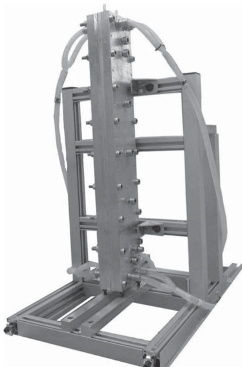
Fig. 1 Thermogravitational column with parallelepiped configuration
