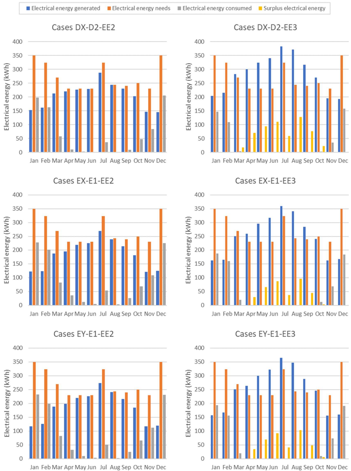
Figure A2. Monthly electrical energy balances for cases EE2 and EE3 in the different CCZs.
