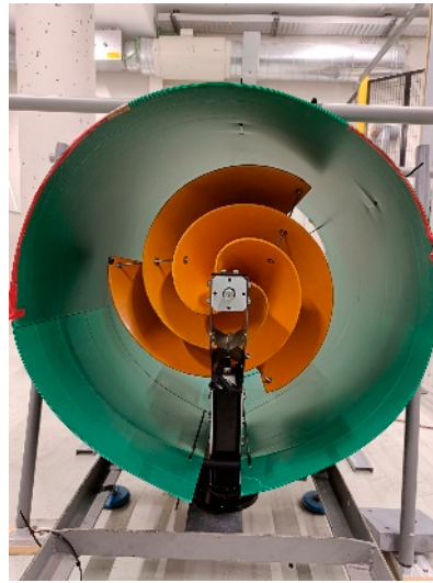
Figure 8. Assembling with a reconfigurable plastic green tube to test the most appropriate longitude and diameter of the tube in terms of power generation.
