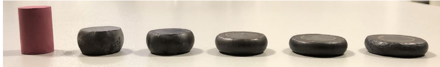
Fig. 2. Initial sample and samples tested in the DIDH at 900°C, 940°C, 980°C, 1000°C and 1020°C (from left to right).
