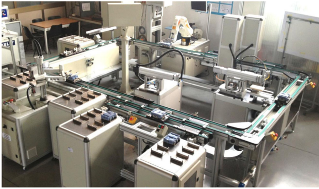
Fig. 7 The ECU Assembly System (MASMEC) [78]
