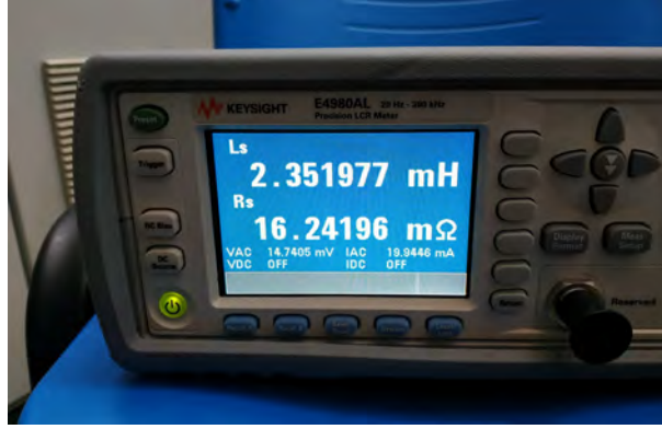
Fig. 5.12. Measurement of the plant parameters L_f and R_f by a LCR meter.
