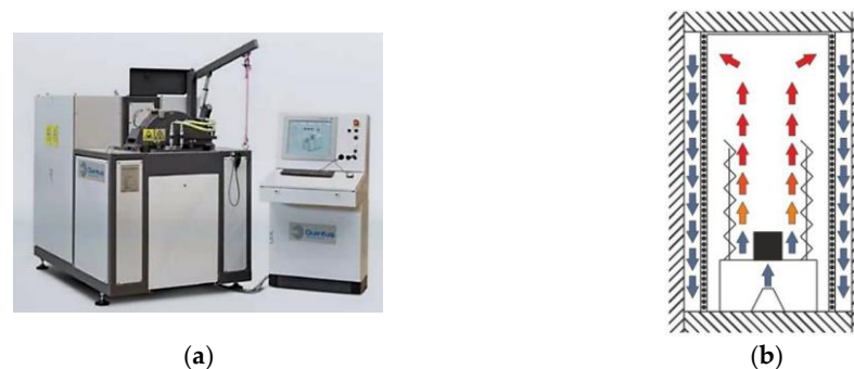
Figure 4. HIP; (a) Quintus-QIH9 model and (b) URQ ® technology.
