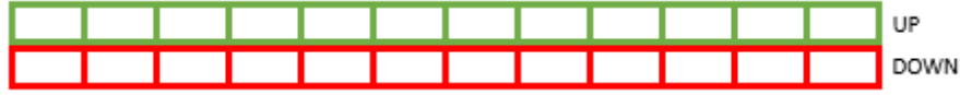
Figure 9. Origin data structure. It contains the number of passengers that have entered any lift at each floor in the last 50 seconds. In this case, it would be a building of 12 floors.
