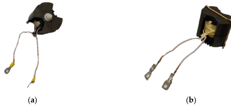
Figure 8. Mounted inductance for the (a) HB ( L = 150 \mu\text{H} and R_L = 26 \text{ m}\Omega ) and (b) MSIBC ( L = 75 \mu\text{H} and R_L = 31 \text{ m}\Omega ).
