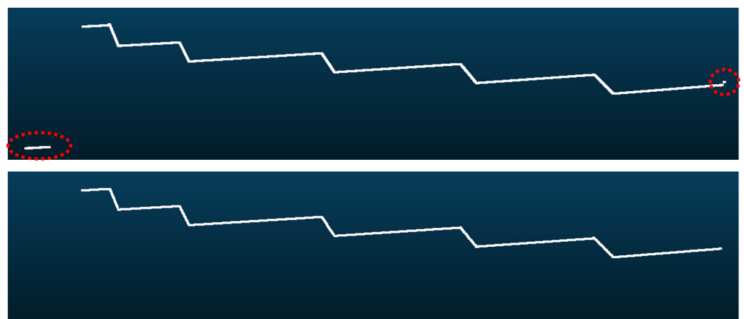
Figure 7. Example of captured laser profile for the calibration pattern. Raw data with noise highlighted in red ( top ), and the result after removing noise and detect lines ( bottom ).
