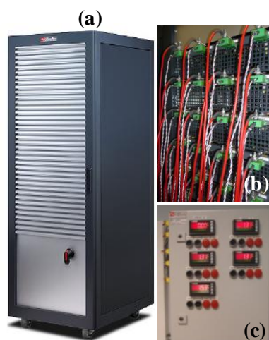
Figure A-11. Digatron MCT cell tester (a), tests circuits in it (b) and safety box (c)
