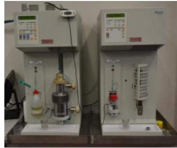
Figure A-22. Thermo Scientific Mercury Porosimeter PASCAL 140 and 440 Series (chemical lab of ISEA-RWTH Aachen University, Germany)
