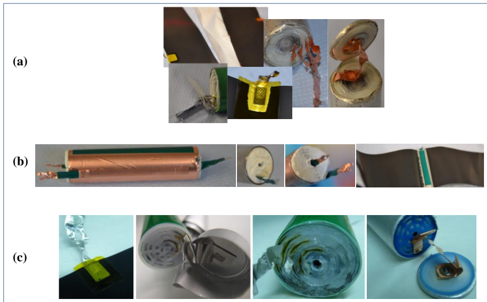
Figure 4-31. Opening of cylindrical cells from three different manufacturers. Cells analysed for the residential elevation application
