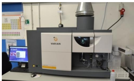
Figure A-24. ICP Optical Emission Spectrometer VARIAN 725-ES (chemical lab of ISEA-RWTH Aachen University, Germany)
