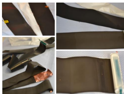
Figure 3-34. Disassembled fresh cells (unused) from different manufacturers
