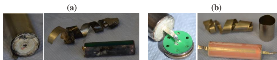
Figure 3-27. Two laptop 18650 aged cells (a and b) cell innards (jelly-roll) extraction
