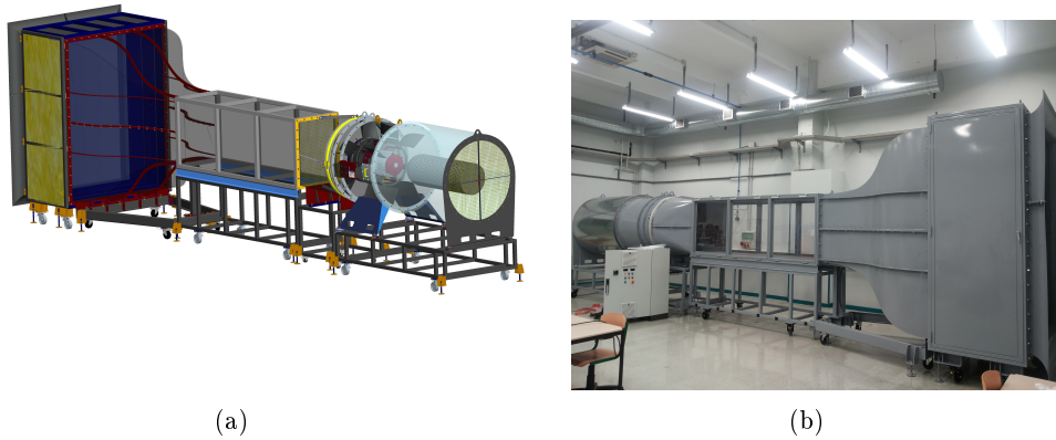
Figure 2.14: LSWT design (a) 3D CAD design (b) LSWT facility installed at MU
