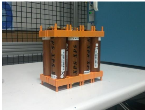
Figure 4.6: 8 cylindrical cell battery module.
