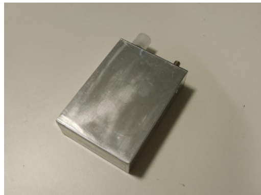
Figure 5.33: 6.5Ah Lishen prismatic power cell.
