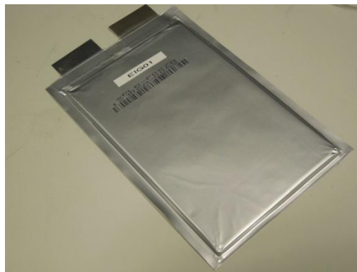
Figure 5.51: EIG pouch power cell.
