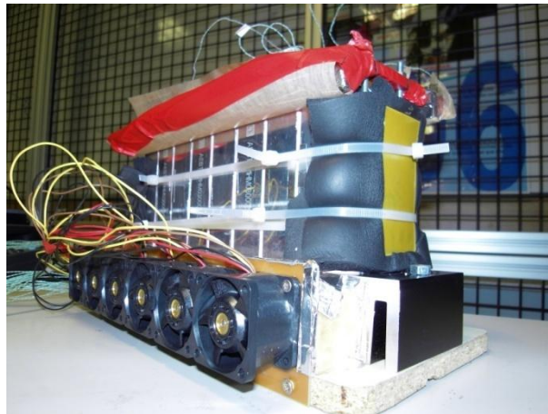
Figure 6.26: Experimental assembly of the prismatic module with the forced air cooling system designed.
