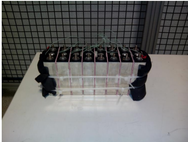
Figure 5.38: Lishen module layout with TIM between cells and thermal insulator materials to match convective heat transfer coefficients.
