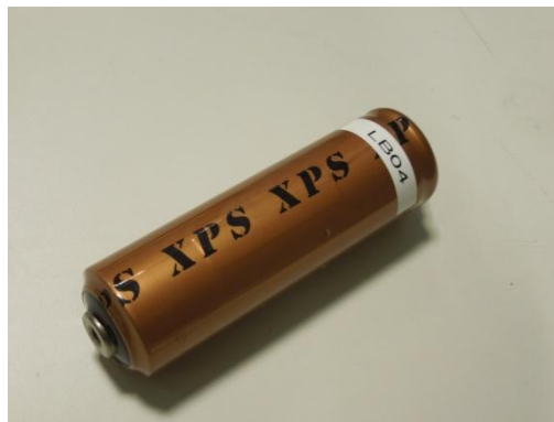
Figure 5.40: LiFePO 4 cylindrical power cell.
