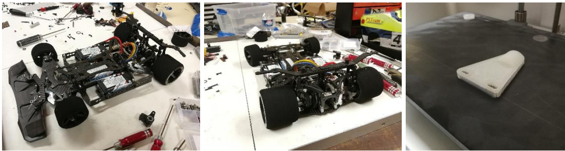
Fig. 9. Carbon fiber prototype with special orientations and a 3D-printed suspension part with nylon honeycomb and fiberglass-fibers (Markforged printer).
