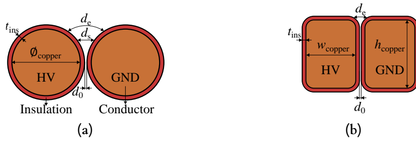
Figure 4.15: Simplified geometries of interturn insulation used in FEM simulations for (a) round conductors, and (b) rectangular conductors.
