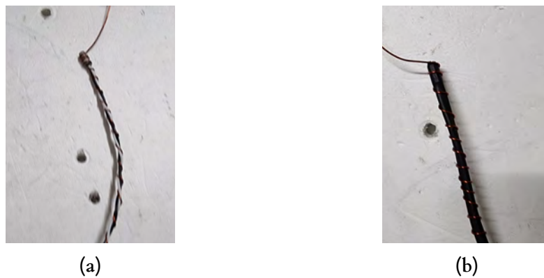
Figure 5.10: Winding wire twisted to the thermistor for PDIV measurements (a) without thermoretractable tube, and (b) with thermoretractable tube.
