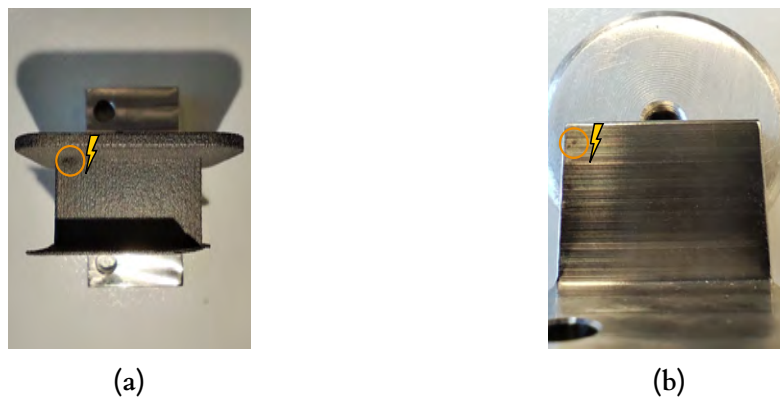
Figure 5.20: Failure location of the breakdown during PDIV measurements of 0.70 mm Nylon 12 sample (a) cap sample, and (b) electrode.
