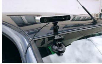
Fig. 4: Camera setup for the recordings of the generated dataset.
