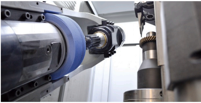
Fig. 1. SG 160 Sky Grind machine work area configuration.
